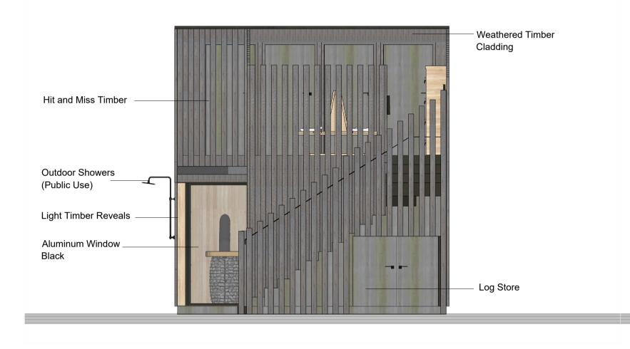
Proposed Sauna West Elevation Scale 1:50 @A1
