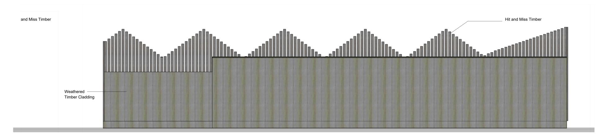
Proposed Toilets and Bin Store North Elevation Scale 1:50 @A1
