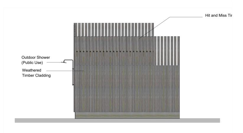
Proposed Toilets and Bin Store West Elevation Scale 1:50 @A1
