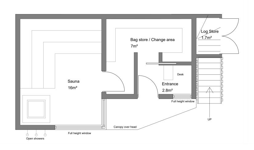
Proposed Sauna Ground Floor Plan Scale 1:50 @A1
