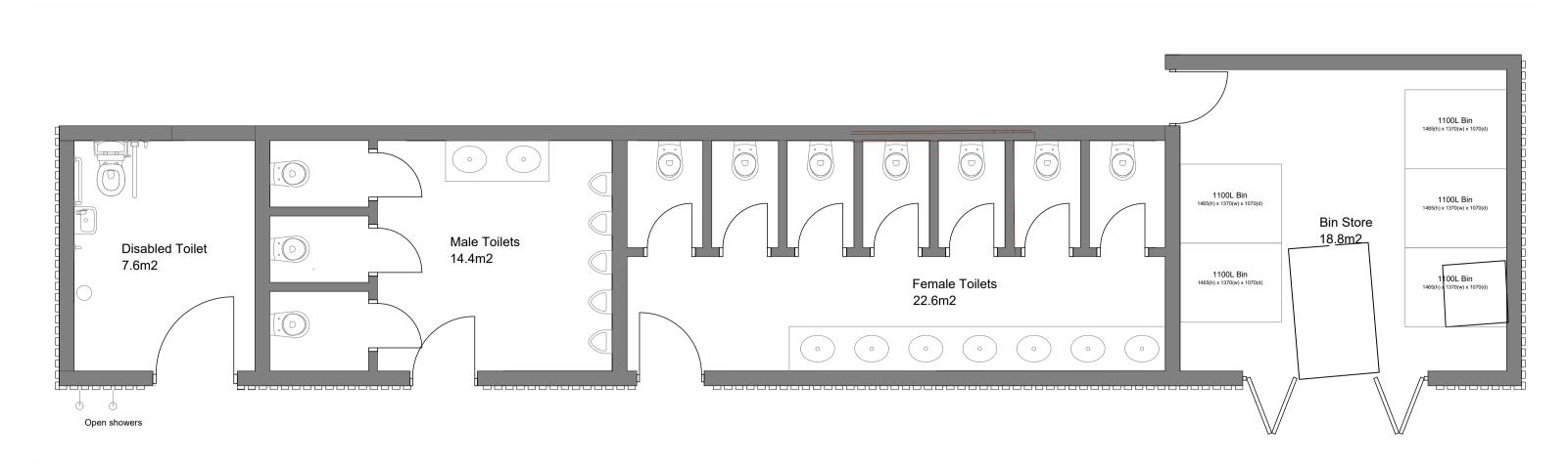
Proposed Toilets and Bin Store Ground Floor Plan Scale 1:50 @A1
